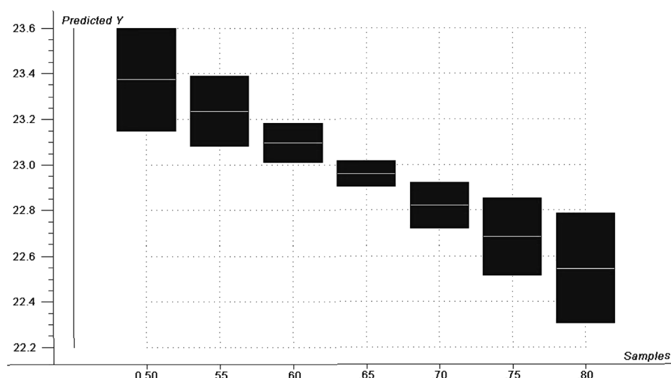
FIG. 11. Predicted variation in the logarithm of the cake resistance ( \ln(x) = y ) from a simulated variation in the porosity with the other x -variables set constant and equal to their mean values.
